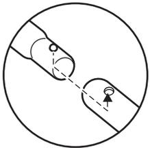
Be sure to lock buttons when fitting tubes together.
